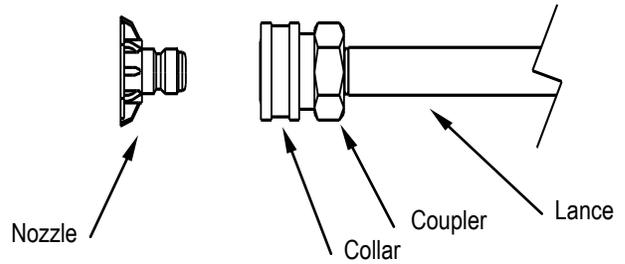
3. Release the collar, making sure it springs back and re-seats to its original (non-retracted) position. Check the connection by pulling on the nozzle to ensure a tight connection -- if correctly inserted, nozzle will rotate but not pull out.
