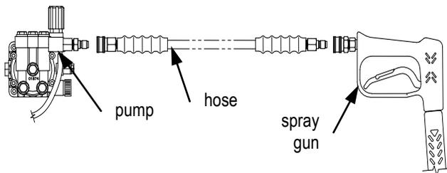
1. Make sure the engine is off and the hose line depressurized.
