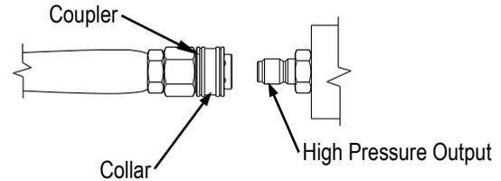
3. Release the collar, making sure it springs back and re-seats to its original (non-retracted) position. *Check the connection by pulling on the hose to ensure a positive connection.*
