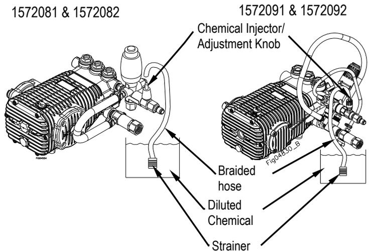
**Note:** Adding accessories (IE: telescoping wands, extra length of High pressure hose, Non factory triggers) will affect chemical injector performance or cause it not to operate at all.
